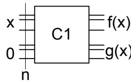
This circuit has  $C_1$  gates and accepts  $n$  bits at the input (including data bits  $x$  and work bits 0).  $g(x)$  is the data loaded on the work space after the operation of the circuit.  $f^{-1}$  can also be constructed using the following circuit with  $C_2$  gates:
