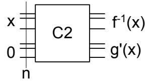
Show that there exists a reversible circuit with the following operation that uses only  $k(C_1 + C_2 + n)$  gates where  $k$  is a small constant:
