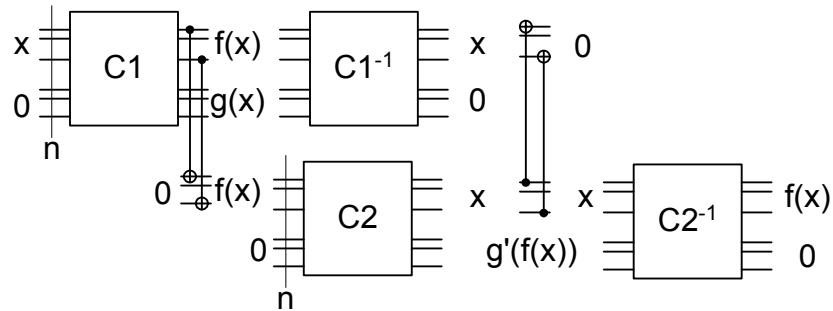
where  $C1^{-1}$  and  $C2^{-1}$  are the reverse circuits to  $C1$  and  $C2$ . The above circuit uses less than  $2(C_1 + C_2 + n)$  gates.
