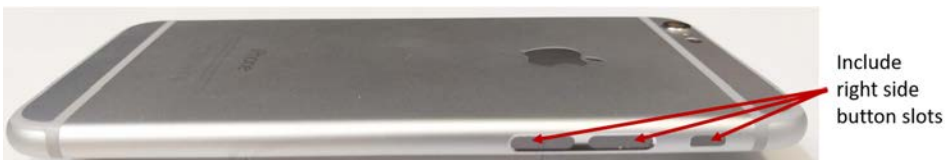
Figure 3: Include right side button slots in the process plan.
