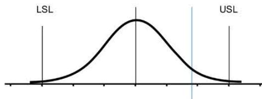
$$C_{pk} = \frac{USL - \mu_x}{3\sigma_x} \quad \text{or} \quad C_{pk} = \frac{\mu_x - LSL}{3\sigma_x}$$
