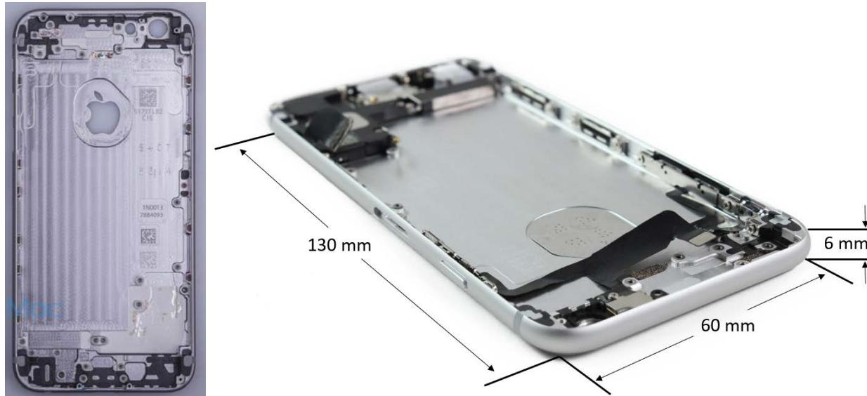
The part material is 6061-T6 aluminum alloy with the following properties:
