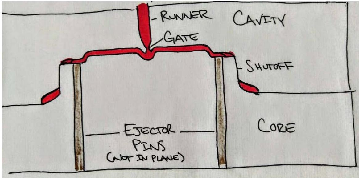
\*Note that ejector pins are not technically in the plane of the section, so OK if not included in the sketch
