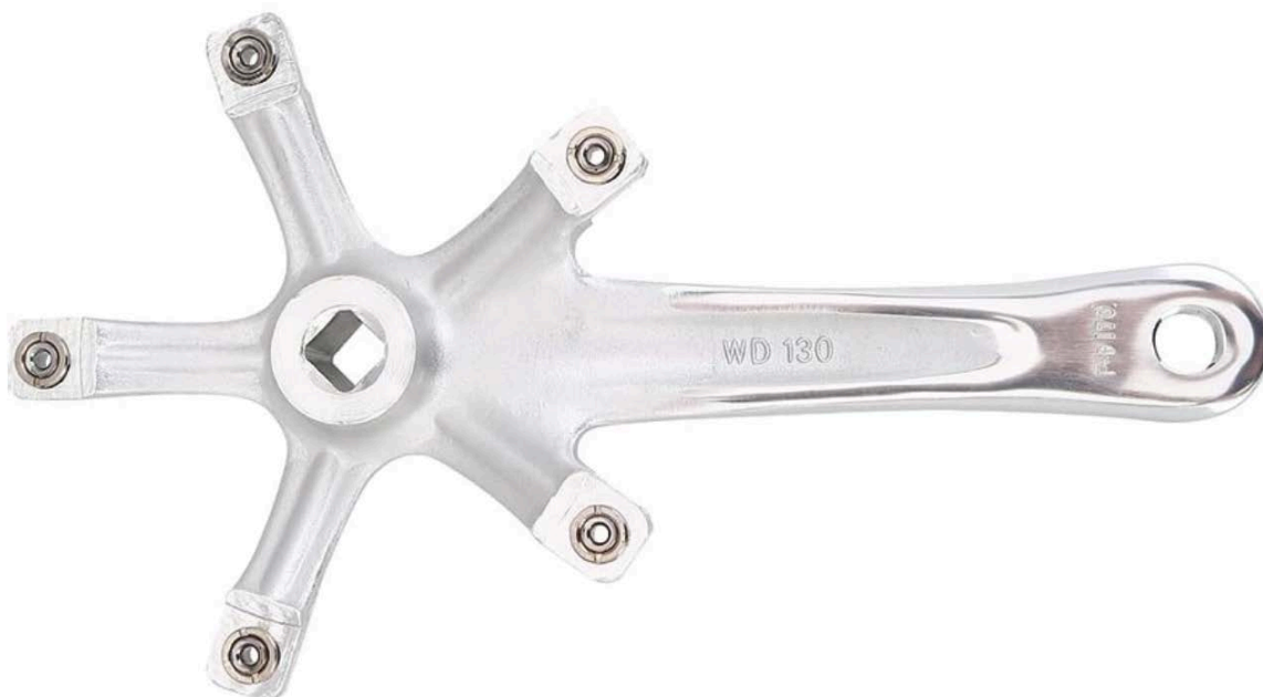
Figure 7: Backside of drive side crank.
