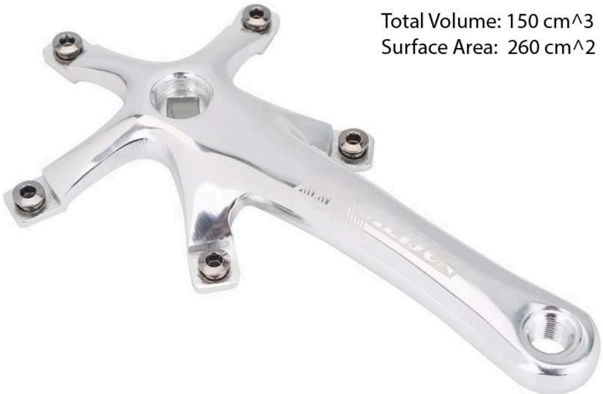
Figure 6: Isometric view of drive side crank.
