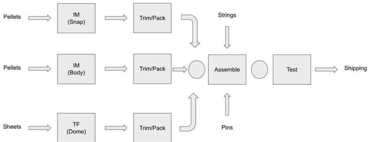
Each box denotes a separate machine and operation on the line. Arrows denote how and which direction the Yo-Yo's move through the transfer line. There are no places for buffers unless a circle is present. The size of the buffers will be changed throughout the different questions below. Materials that are used within the machines/operations are denoted with text and do not constitute an operation themselves if not boxed.
