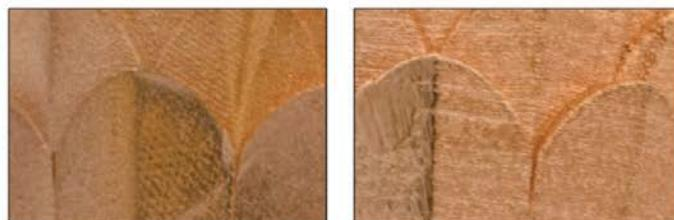
The rate limiting step or bottleneck in this problem was the grinding step and the image shows that the 3D printed wax molds still process visible linearization, so the grinding and finishing process will still need to take place in order to produce desired part finish. This means the for the customer likely with a similar operation time. It is possible that the Traditional casting of the 3D mold can help retain some of the finer detailed features.
