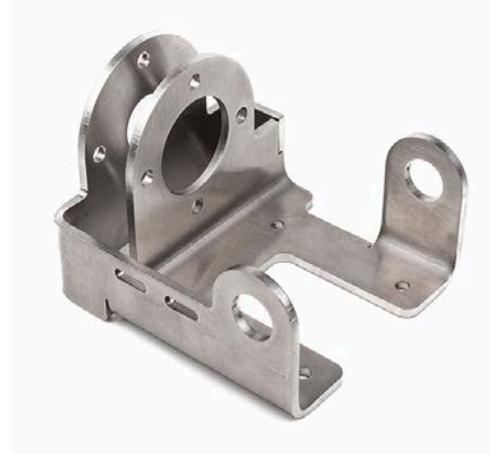
For the questions below, we will ignore the cut holes and focus on the bracket itself, which is made with sheet metal bending. The panel is 4mm thick, and during bending operations, the initial radius of curvature is 10mm.
