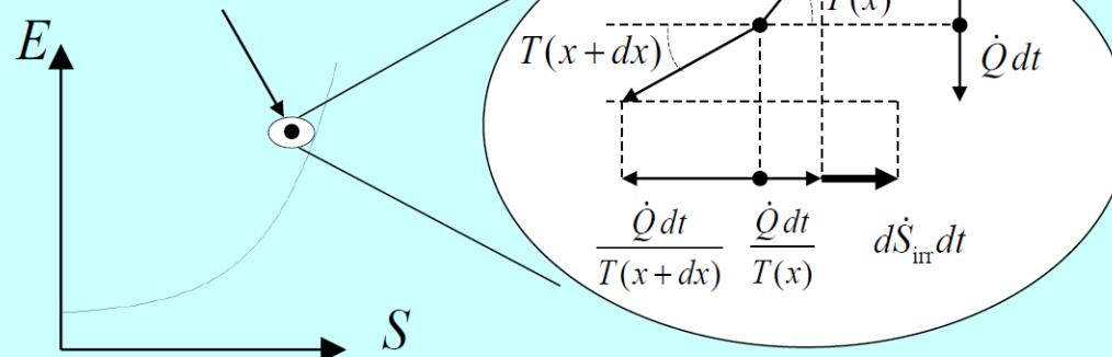
$$\begin{aligned} d\dot{S}_{\text{irr}} &= \frac{T(x) - T(x+dx)}{T(x)T(x+dx)} \dot{Q} \\ &\approx -\frac{dT}{dx} \frac{\dot{Q}}{T^2} dx \end{aligned}$$
