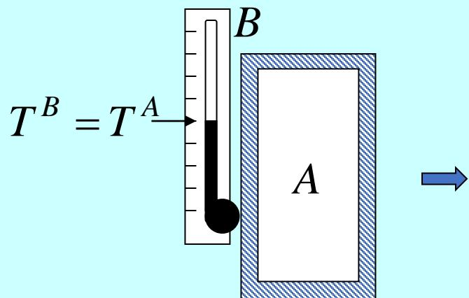
The temperature read by thermometer  $B$  is equal to that of system  $A$ , regardless of the details of system  $A$ .
