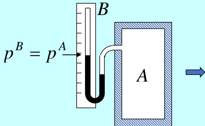
The pressure read by manometer  $B$  is equal to that of system  $A$ , regardless of details of system  $A$ .
