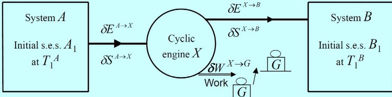
Energy and entropy balances for  $X$ ,  $A$  and  $B$  (assuming **reversible** processes), and Gibbs relations for  $A$  and  $B$ :
