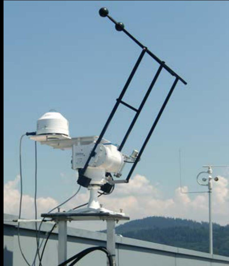
Tracking Pyranometer on the roof of the Fraunhofer ISE
