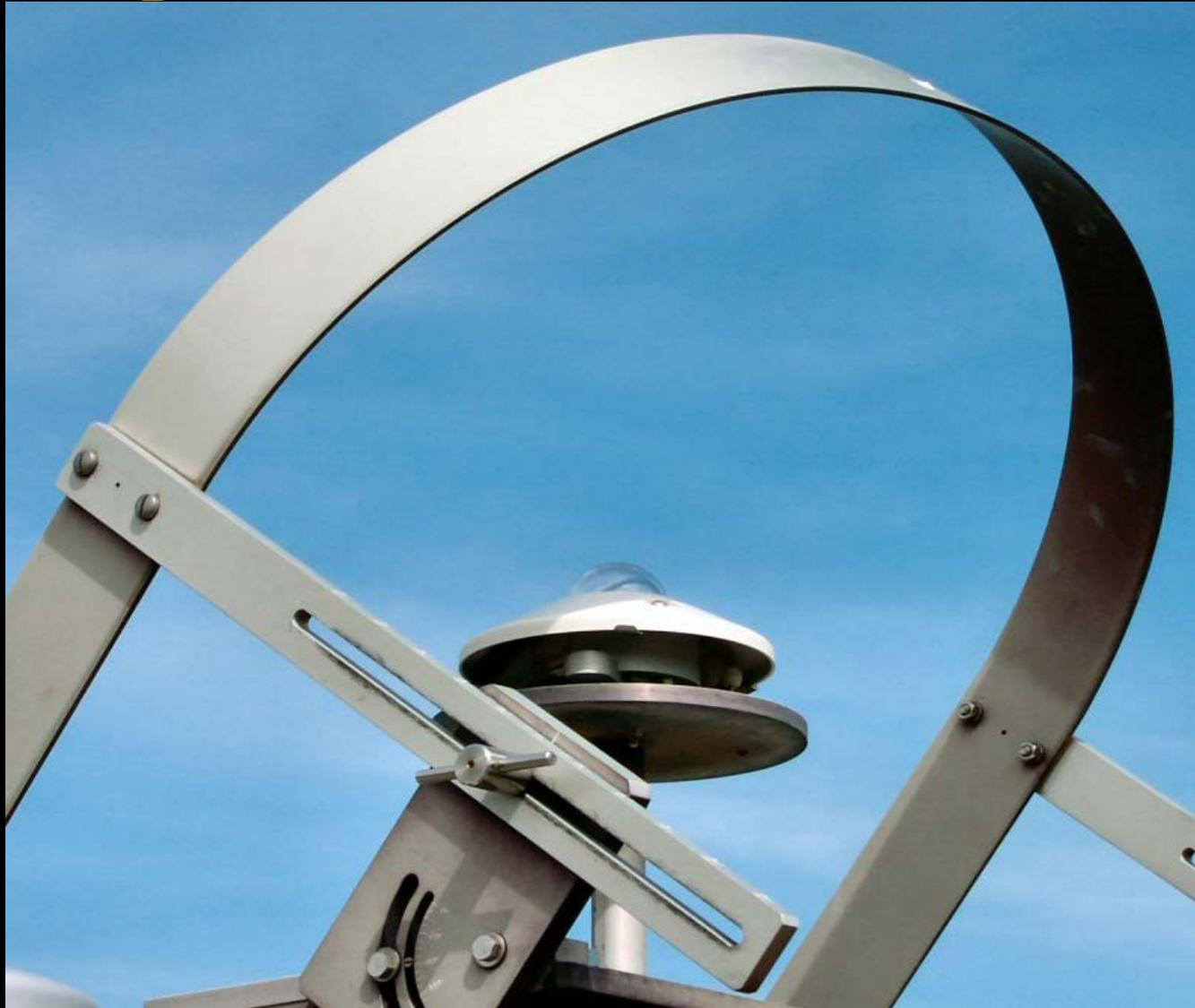
Shadow band pyranometer
